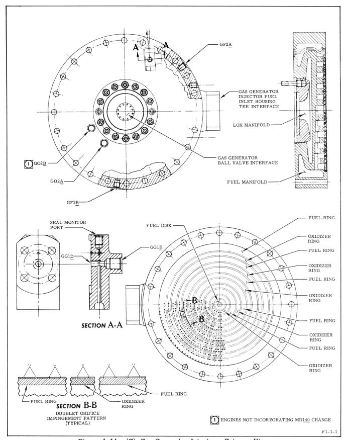
Figure 1-14. (C) Gas Generator Injector--Cutaway View
