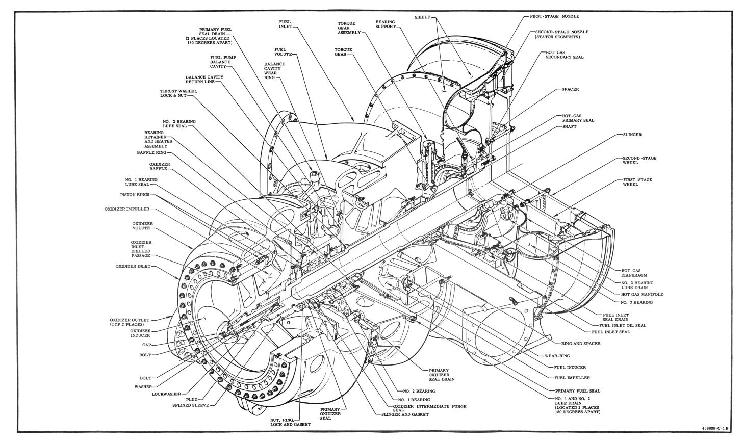
Figure 1-30. (C) Turbopump--Cutaway View
